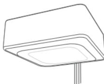
**IMPORTANT:** For best range results, we recommend mounting the E1000 on the ceiling in an unobstructed location.
