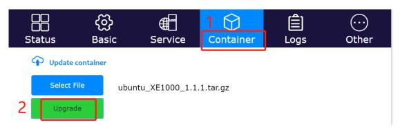
Now, the container will be uploaded and installed on the gateway.
