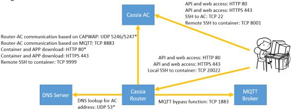
Please make sure the following ports are opened outbound on the gateway side firewall. The user can check if a TCP port is opened by using Netcat in gateway's local console.
