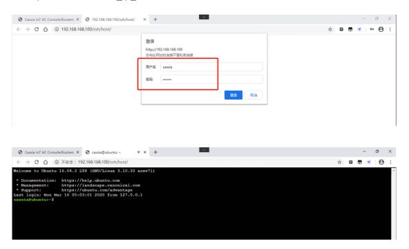
After logging into the container with SSH, the user can control Bluetooth with RESTful API, noble, or dbus. Users can also use apt-get command to install Linux tools. For example, the user can run "apt-get install Irzsz" to install Irzsz.
