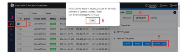
From firmware 2.0, a new tab will pop up on the web browser as an SSH terminal. After pressing the "Remote Login" button, the user can still log in to the container by "ssh -p 8001 cassia@ac\_ip\_address" in other terminals.
