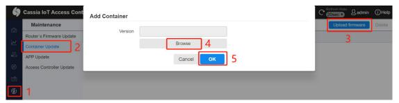
Second, please follow the steps on the AC console to install a container to a batch of gateways: Gateways->select the gateways that need to install Container->More->Container->Install.
