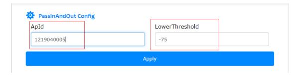
After the configuration, the gateway will generate file config.json under folder /root/config/<app\_name>/.
