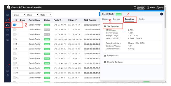
The user can also delete, reset, start, stop, and remote login containers from the AC. Please follow the steps on AC console: Gateways ->select gateway->Edit->Container->Operate Container
