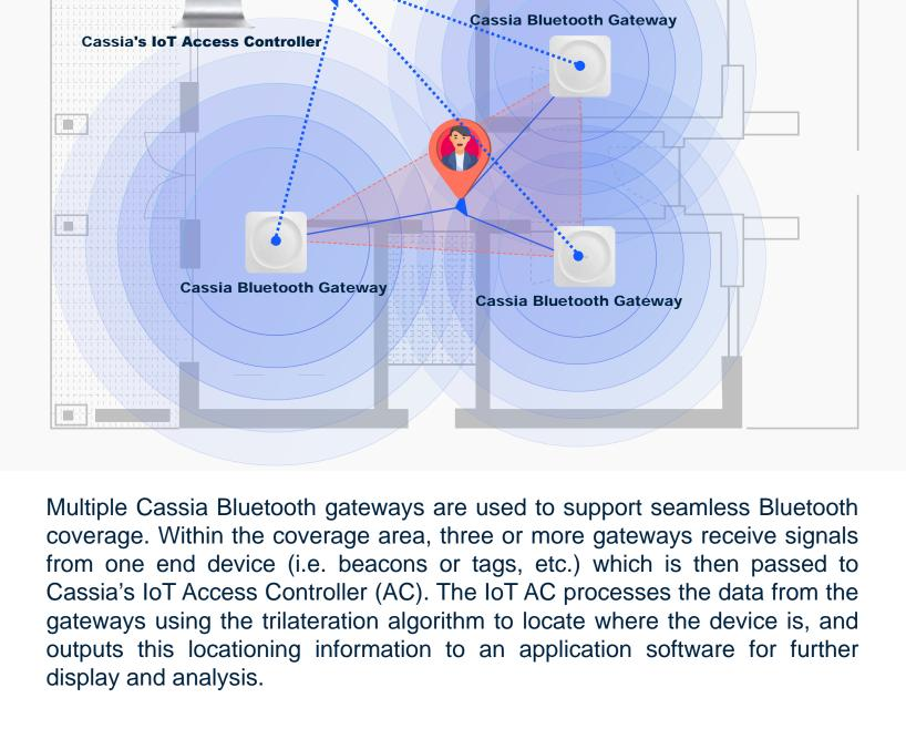
MachinesTalk is using Cassia's Bluetooth IoT products and solutions to provide personnel & asset tracking for Aramco's office campuses
